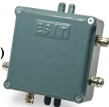
ESIT-J It is lightning protected, resistant to water, aluminum cast and Ex-proof housed.
